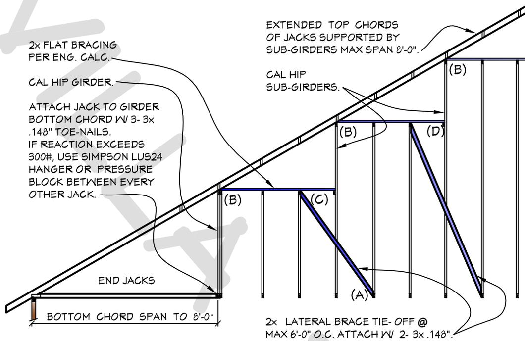
WHERE TWO MEMBERS MAKE CONTACT, MIN 2- 3x .148" MUST BE USED TO CONNECT EACH MEMBER TOGETHER.
